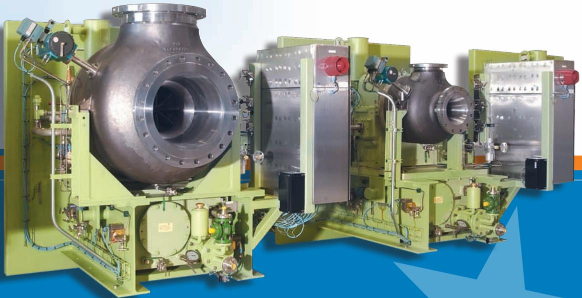
Electric motor driven single stage cryogenic compressor, type CM, with adjustable inlet guide vanes, complete with lube oil system, seal gas system, and accessories. The whole unit is installed on a single, rigid skid, with bulkhead, and bulkhead seal mounted to the heavy-duty gearbox. Typically this machine delivers up to 40,000 m<sup>3</sup>/h of boil-off gas with an inlet temperature of -140°C.
